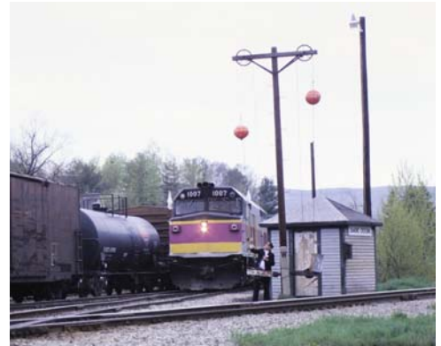
Mass Bay RRE's Day White Mountains excursion pauses at the ball signal in Whitefield on May 16, 1982, as the conductor lines the signal for the B&M main line. (Photo by Len Bachelder)
